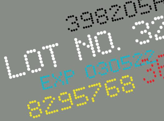
Pigmented inks provide contrast codes across a wide array of substrate colours. Using continuous inkjet printing with pigmented inks, you can:
